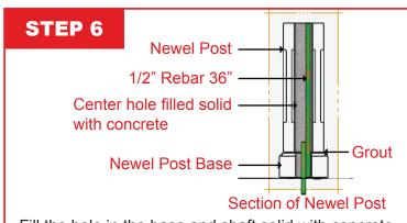
Fill the hole in the base and shaft solid with concrete and insert 1/2" rebar in filled hole through the base and shaft. *Tip: Grout joint between base & shaft prior to filling*
