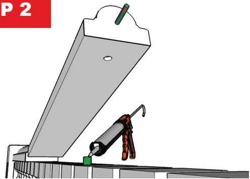
Each handrail should be doweled to one another following the same steps you did for the handrail to the newel post. Additionally, the handrail should be doweled to 1 baluster for each section of handrail.
