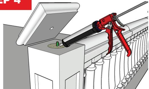
Finish each newel post by drilling a 1" hole on the under side of the cap and secure it to the post using concrete adhesive. The cap should sit over the rebar that protrudes from the top of the newel post. This will lock the cap onto the newel post shaft.
