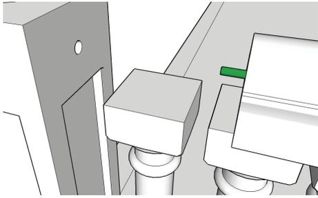
Laying out of the handrail should be done prior to installing any pieces. Some cutting may be necessary to install pieces equal/equal. Never leave a 2" piece.
