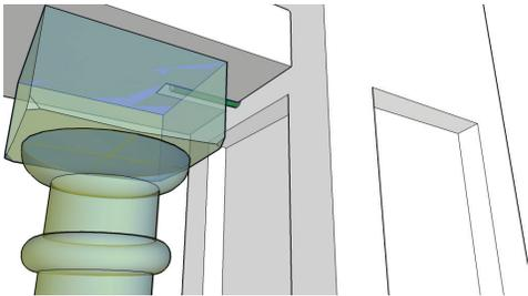
**Repeat step #2** for each section of handrail. The final piece of handrail should be notched at the end, so the handrail sits on the dowel which is inserted into the newel post first. Now all your components are not only "glued" together, but mechanically fastened.
